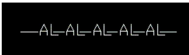
If we put this into words, we would be saying, "Draw a line 1 unit long, lift the pen for 0.25 of a unit, then add "AL" as text using "STANDARD" font style, now lift the pen for 1.25 units, and then repeat the process".
